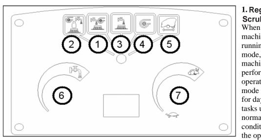
1. Regular Scrub Mode When the machine is running in this mode, the machine will perform all operations. This mode can be used for day-to-day tasks under normal conditions. When the operator sets
