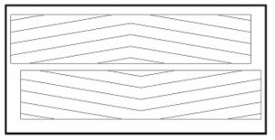
Cylindrical scrub brushes must be installed with the chevron pattern pointing away from each other for best water and debris pick up.
